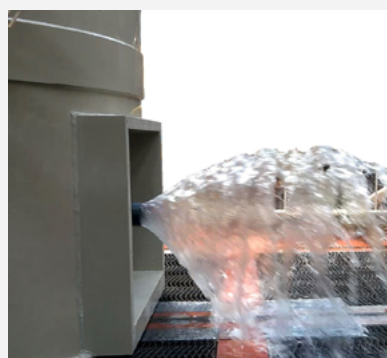
Validation of outflow as a function of water height using a data acquisition system. A limiter is installed in the tank. The formation of the air cone is visible at the outlet (vortex effect).
