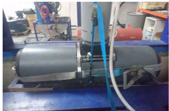
Tightness and pressure resistance tests on NORHAM's test bench.
