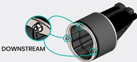
b) To install it **UPSTREAM**, remove the plate fasteners.
