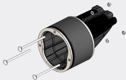
b) The check valve is ready to be installed **UPSTREAM** of the pipe.
