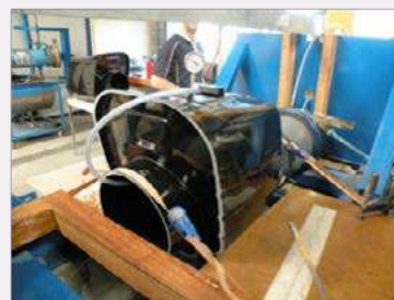
Validation of the pressure resistance of a MULTI 315 valve. The same type of test is applied to all valves in the MULTITUBE range.
